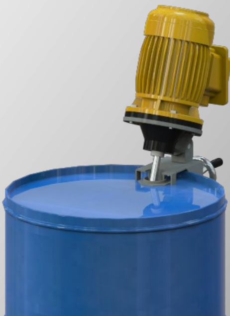
Above: Drum clamp mixers feature a locking mechanism specifically designed to fit standard 205L drum bungs. The quick release screw clamp makes removal quick and easy. A folding impeller allows the mixer to suit small diameter bungs.
