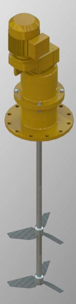
**Above**: Standard top entry mixers consist of a gearbox and motor assembly, single or multiple pedestals, a shaft and single or multiple impellers.
